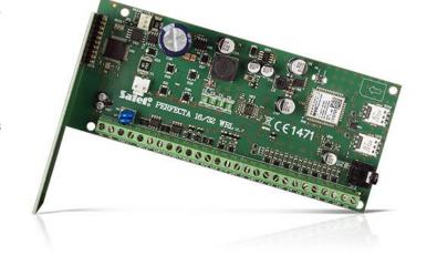
supported to ensure continuity of communication: if any problems occur with the first operator range, the second card is automatically selected.
